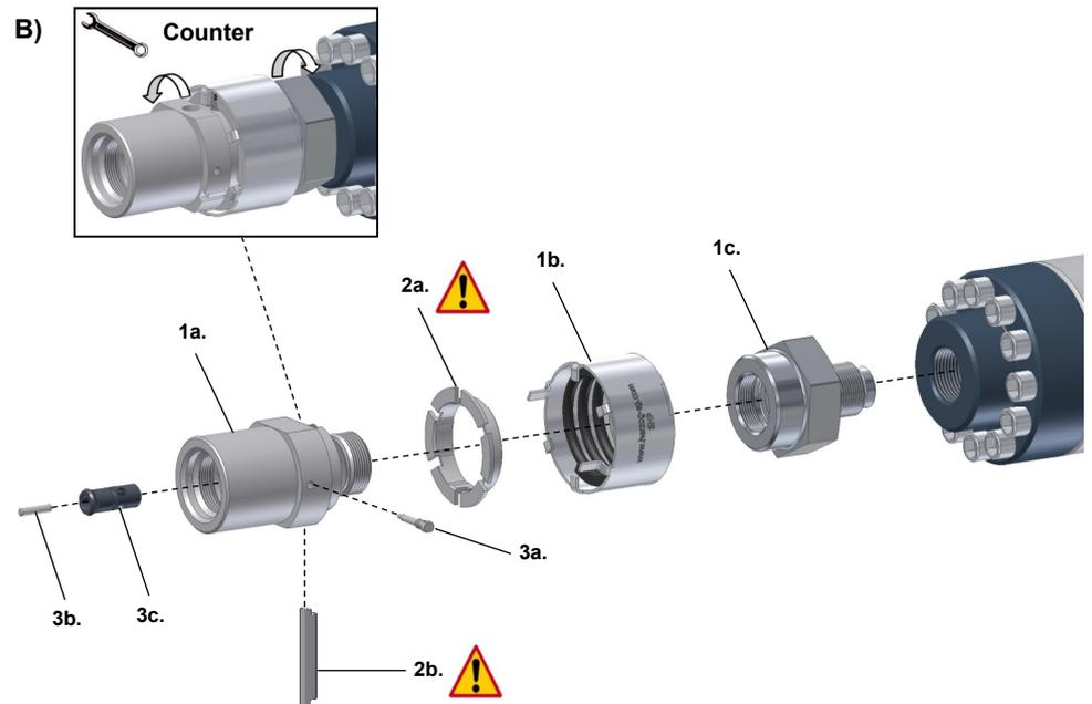
1. Remove body (1a.), spring package (1b.), and adapter (1c.)
